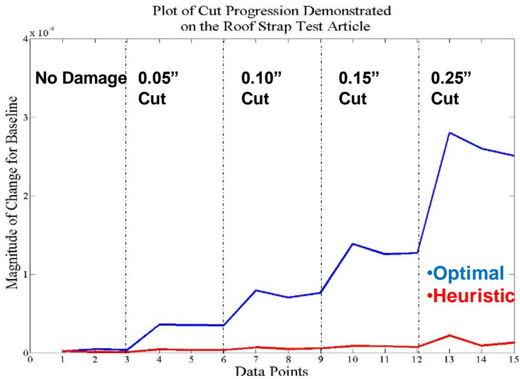
Figure 1. Results of the Cutting Demo on Kiowa Warrior Roof Strap
