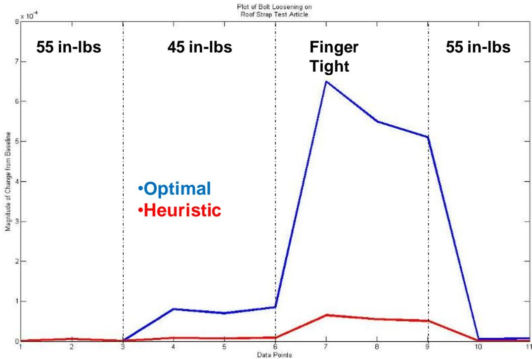
Figure 2. Results of the Bolt Loosening Demo on Kiowa Warrior Roof Strap
