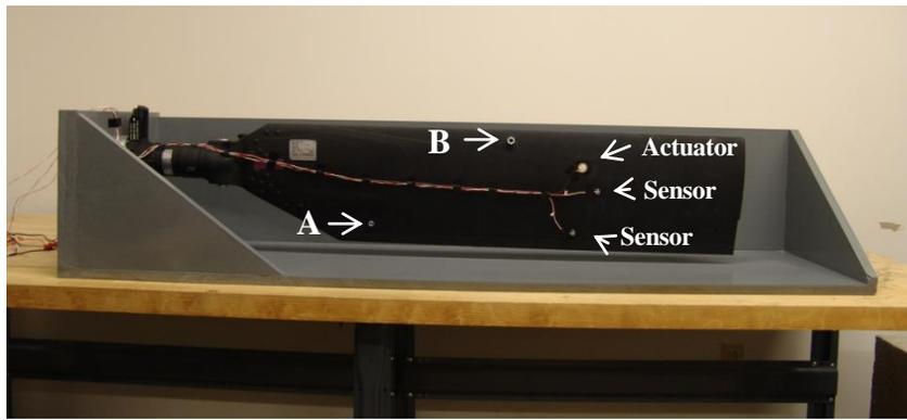
Figure 4. Test Assembly of Tail Rotor Blade – Front View
