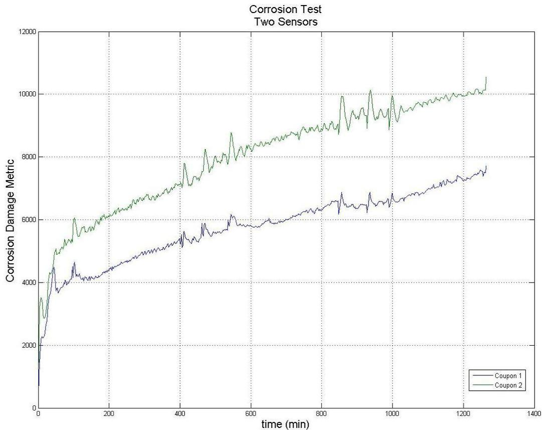
Figure 7. Damage Metric vs. Time for Coupons in Salt Fog Chamber
