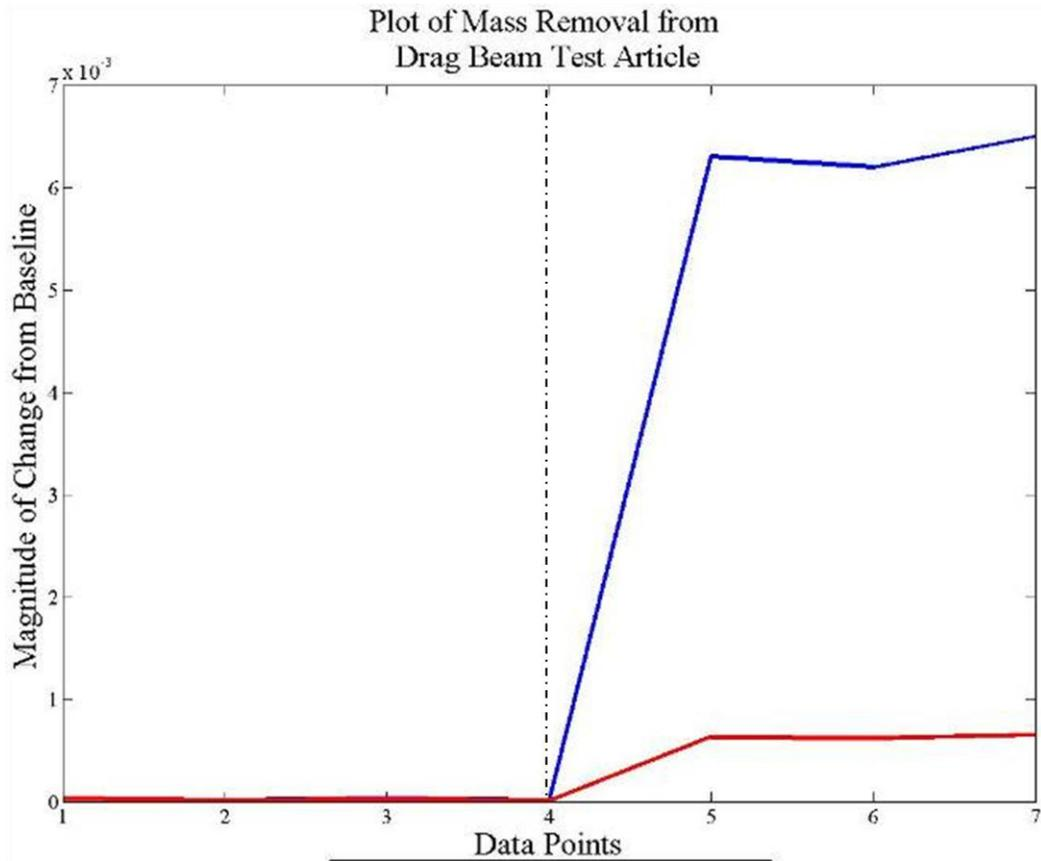
Figure 3. Plot of Damage Detection on the Black Hawk Drag Beam. Optimal in blue, Heuristic in red
